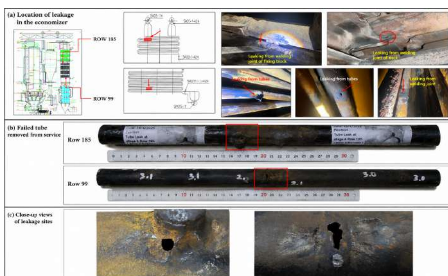
Figure 1. Field inspection and macroscopic appearance of failed economizer tubes.
