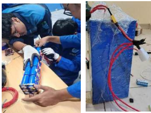
Figure 1. IOT-based Li-Ion Battery pack module
