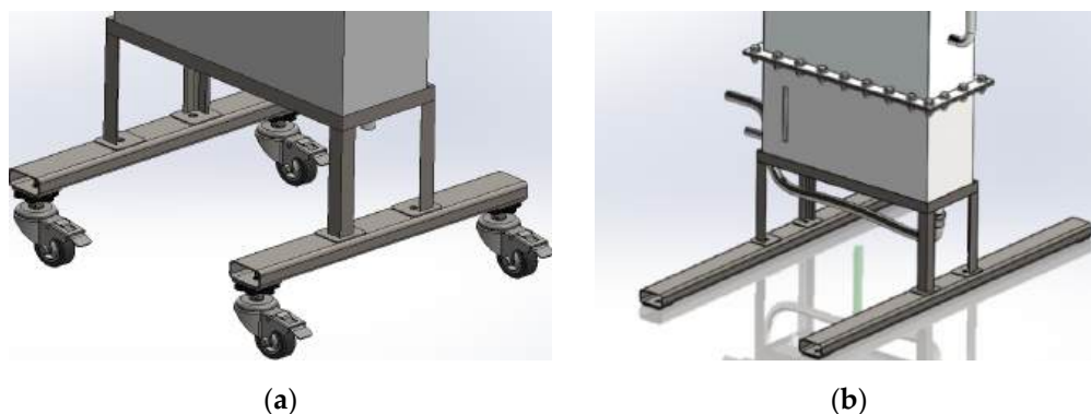
Figure 4. (a) Condition of the leg design before modification and (b) after modification
