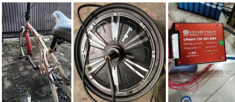
Figure 3. A bike frame, motor hub and Battery Management System.
