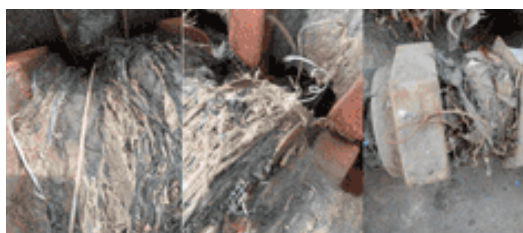
Figure 1. Dynamic disc screen is damaged
