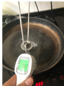
Figure 13. Testing the thermostat at 78 °C temperature
