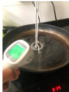
Figure 14. Testing the thermostat at 80°C temperature
