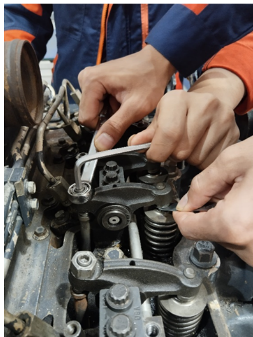
Figure 8. Adjust Valve Lash
