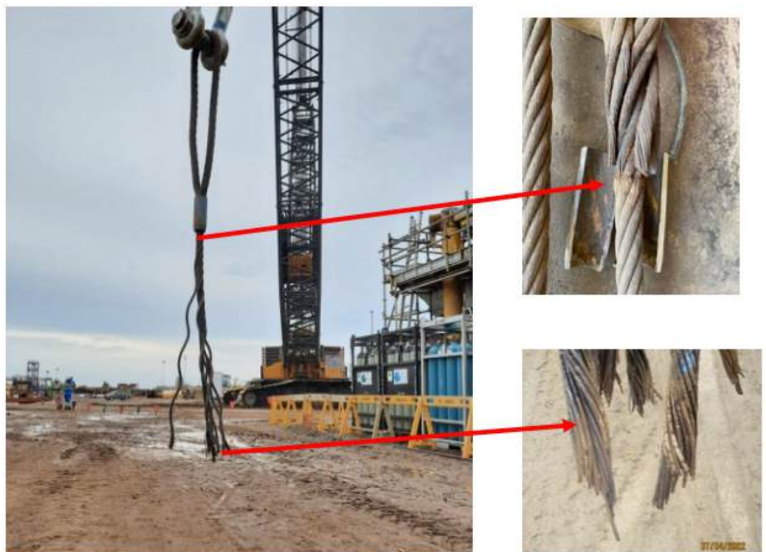
Figure 4. The other end recoiled toward the crane hook. The failure occurred at the sling's ferrule (socket) where the wire rope is swaged, later found to contain corroded wires.
