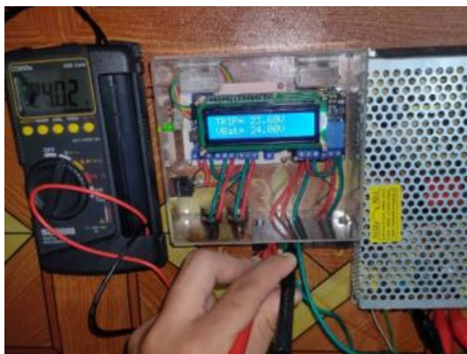
Figur 9. Voltage value reading test with 24V PSU
