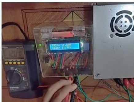
Figure 8. Voltage value reading test with 12V PSU.
