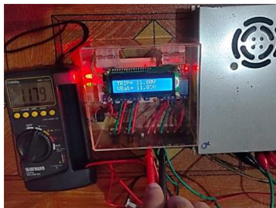
Figure 10. Undervoltage Breaker Trip Execution Testing
