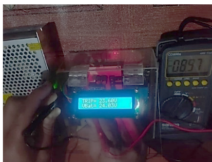
Figure 6. Testing the LM7809 IC as an Arduino Nano supply
