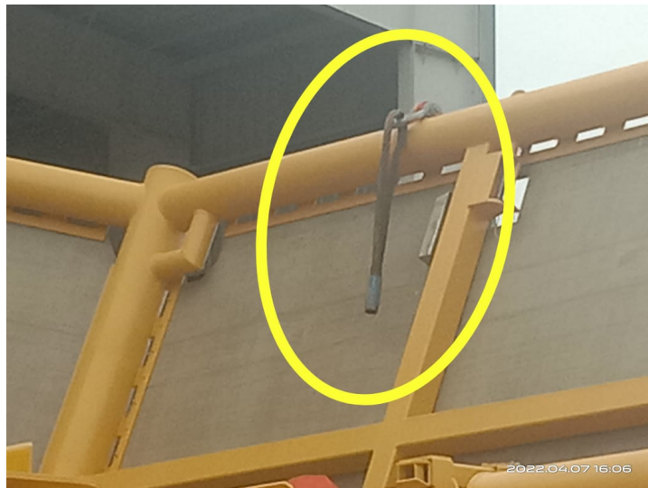
Figure 3. The wire rope sling parted near its end termination – one frayed end remains attached to the panel's padeye (yellow circled).
